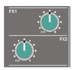
Each Mono Channel on the X-Panda has two mono FX sends (FX1 and FX2)
